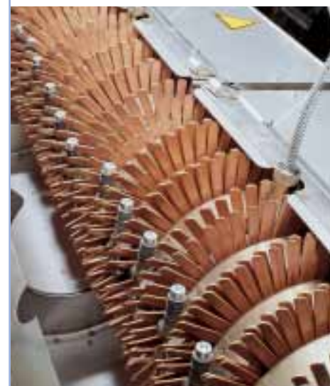
Barrel air cooling system
