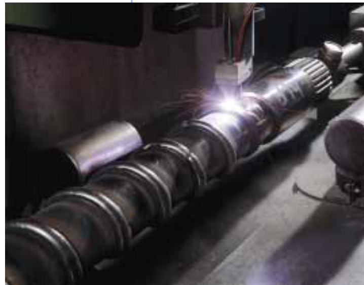
Welding of flights
